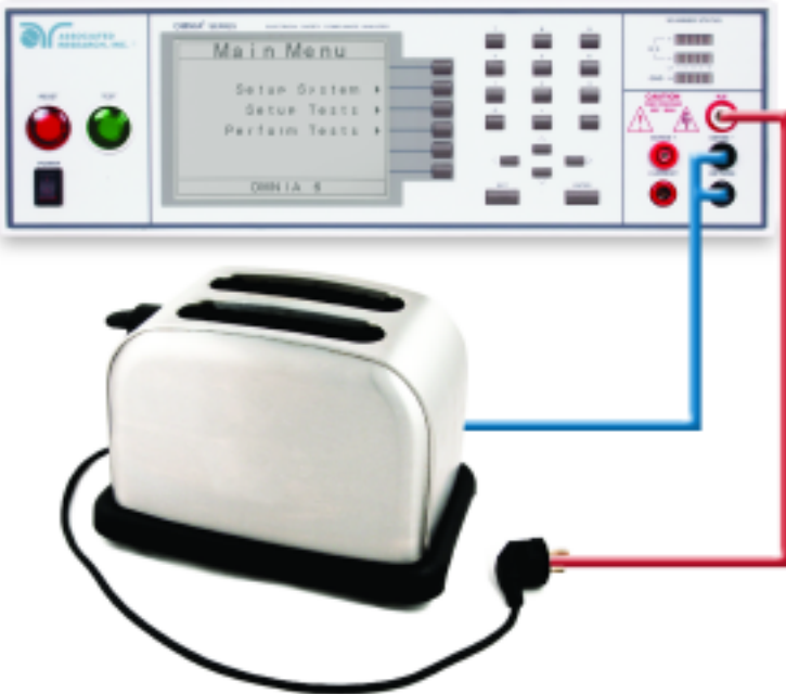
(Figure 6, Test Lead Connection)
